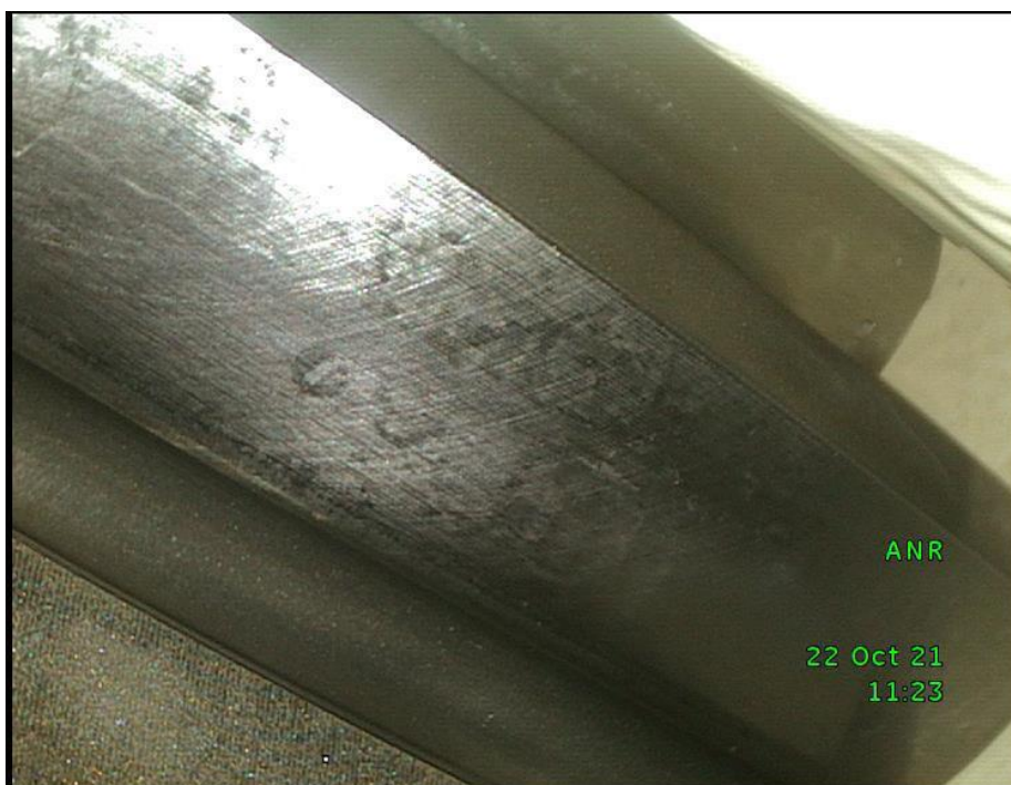
The planet wheels show a lot of irregularities on the surface.
