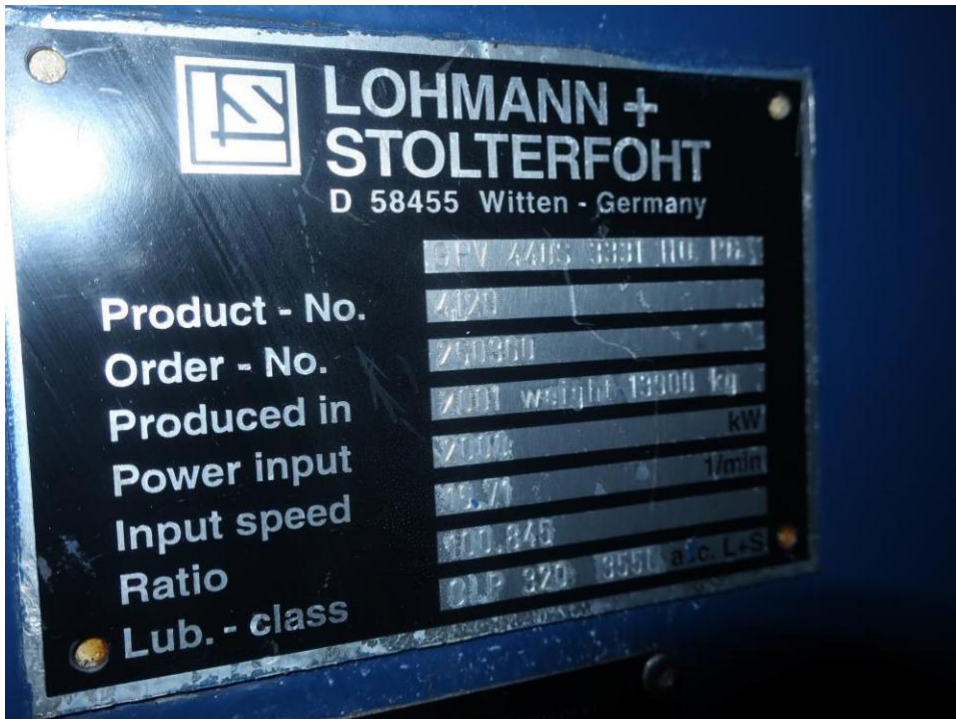
Sign plate of the gearbox.
